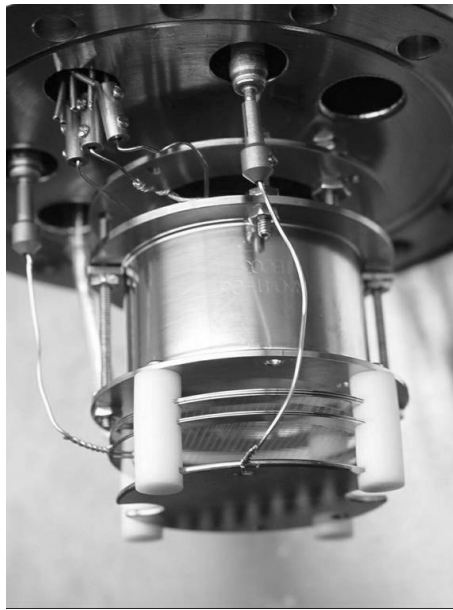
Figure 4.1: Photo of the inner structure of the dual phase chamber. From the bottom are: cathode disk, grid and anode meshes. The Hamamatsu R6041 PMT is mounted above the anode mesh.
