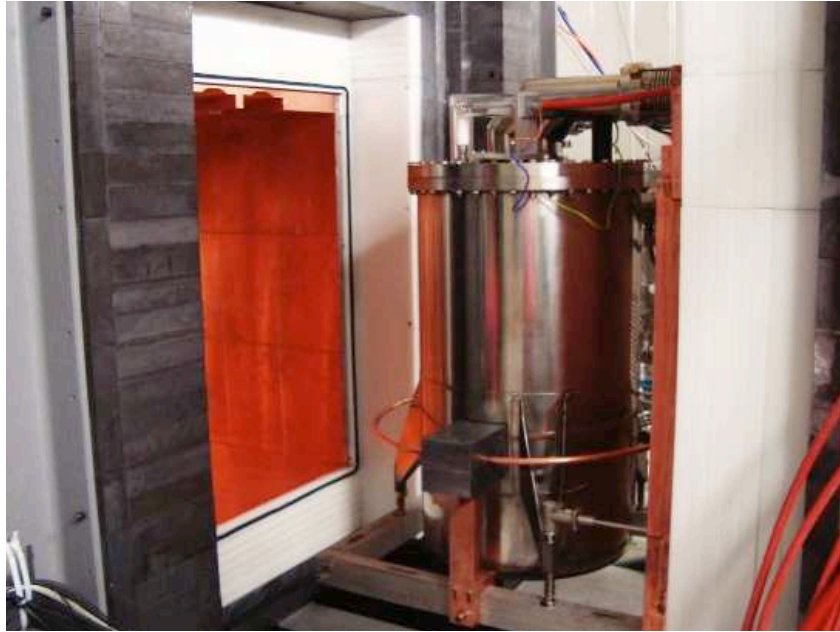
Figure 2. XENON100 after cleaning the cryostat and the shield cavity from dust, grease, stains, etc. right before closing the shield. The circular copper pipe around the detector is used for the insertion of calibration sources from outside the shield. The Pb brick visible in the front is necessary to block gamma rays from the AmBe source during a neutron calibration.
