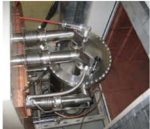
FIG. 58 The XENON100 detector installed in its shield (Aprile, IDM08 Proceedings).
