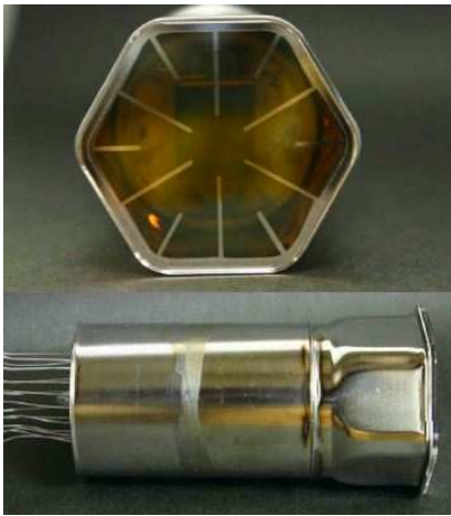
FIG. 64 The hexagonal PMT of the XMASS detector.
