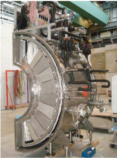
FIG. 76 Image of the full scale MEG LXe scintillation calorimeter.
