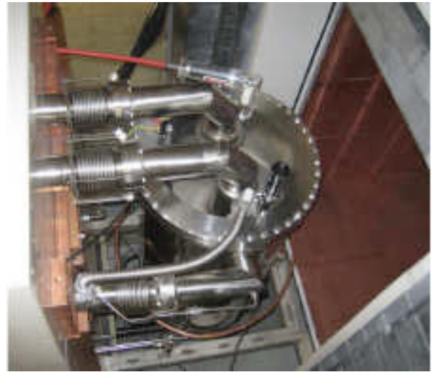
FIG. 58 The XENON100 detector installed in its shield (33).
