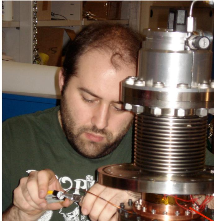
*Pulse Tube Refrigerator (160 W) for Xe liquefaction and Xe gas recirculation*
