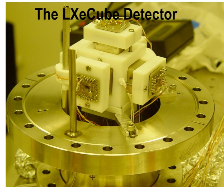
Single-phase LXe scintillation detector, optimized for maximum light collection (>95%): 6 square PMTs detect light from a cube of LXe: 25 pe / keV.
