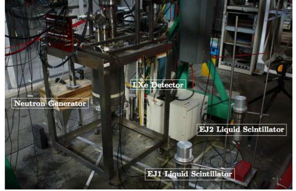
FIG. 5: The measurement principle for neriX using a neutron generator. Neutrons elastically scatter within the LXe detector, and are then detected by two organic liquid scintillators at fixed angles. [3]
