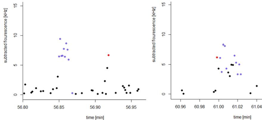
**Figure 5:** Two plots that exemplify the plots I used to analyze the different peak identification methods. The red dots indicate peaks or parts of peaks that the method did not catch. I continued trying different methods until I generated plots that did not contain any red points.
