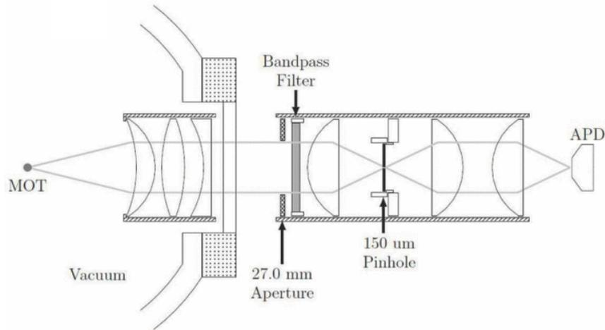
**Figure 2:** The detection setup used to reduce background light and detect the fluorescence of the trapped atoms. Image from: [1]
