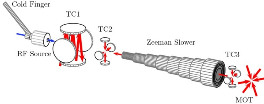
**Figure 1:** This is a diagram of the ATTA system at Columbia University. It shows the setup of how the atoms pass through a plasma created by the RF source, are slowed by the transverse cooling stage and Zeeman slower and then captured in the MOT. Image from: [1]
