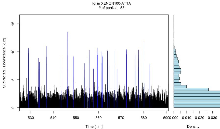
**Figure 6:** Plot of the subtracted fluorescence with the peaks highlighted in blue. Along the side of the plot is a histogram of the peaks that can be used to determine how many atoms were in the trap during a peak. The plot of the subtracted fluorescence is only over half of the time of the trial, while the histogram and number of peaks found are over the whole trial.
