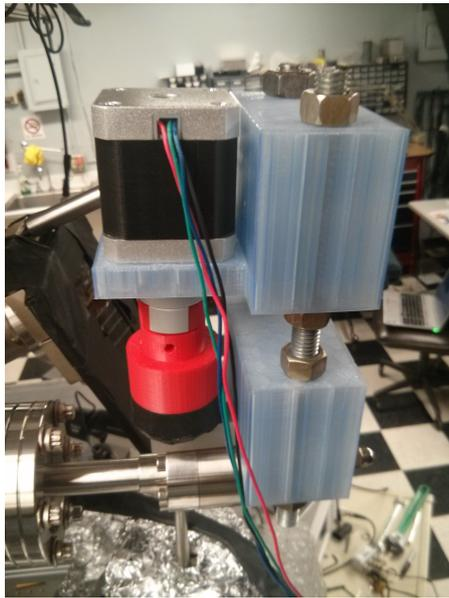
(a) Side View of Pressure Valve Automation
